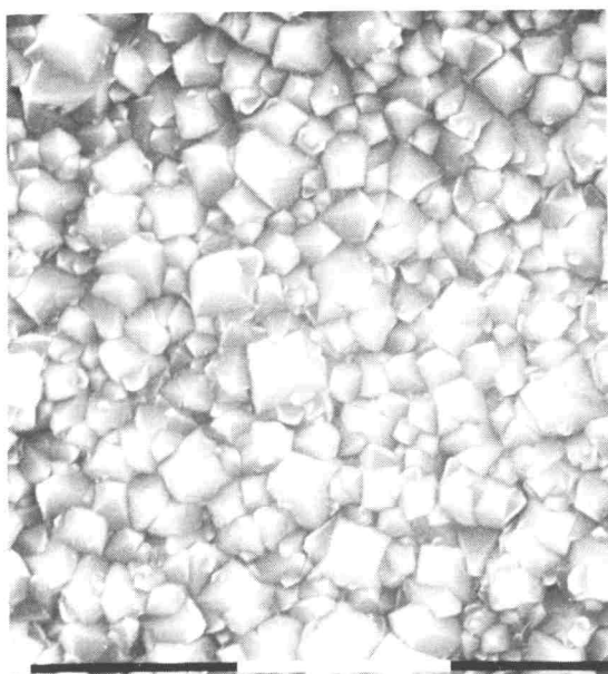
Figure 6 : SEM image of polycrystalline diamond coating produced by the CVD-synthesis (bar length 10 \mu m).
